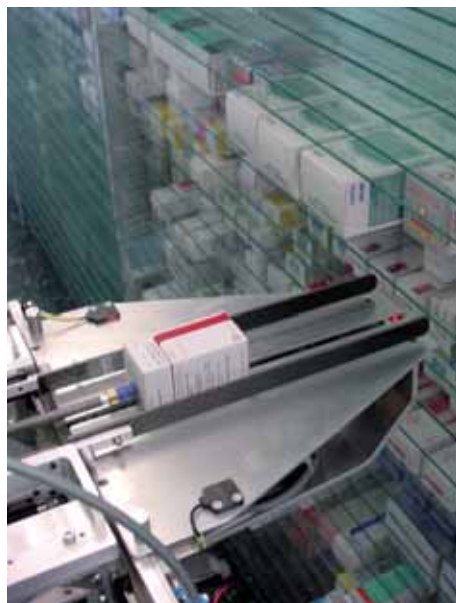
Installation of automated dispensing devices can reduce the storage space required in the dispensary
