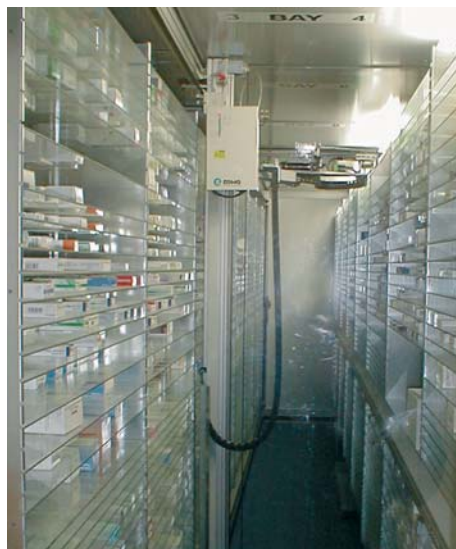
Dispensing robot in place at one branch of Grays Pharmacy
