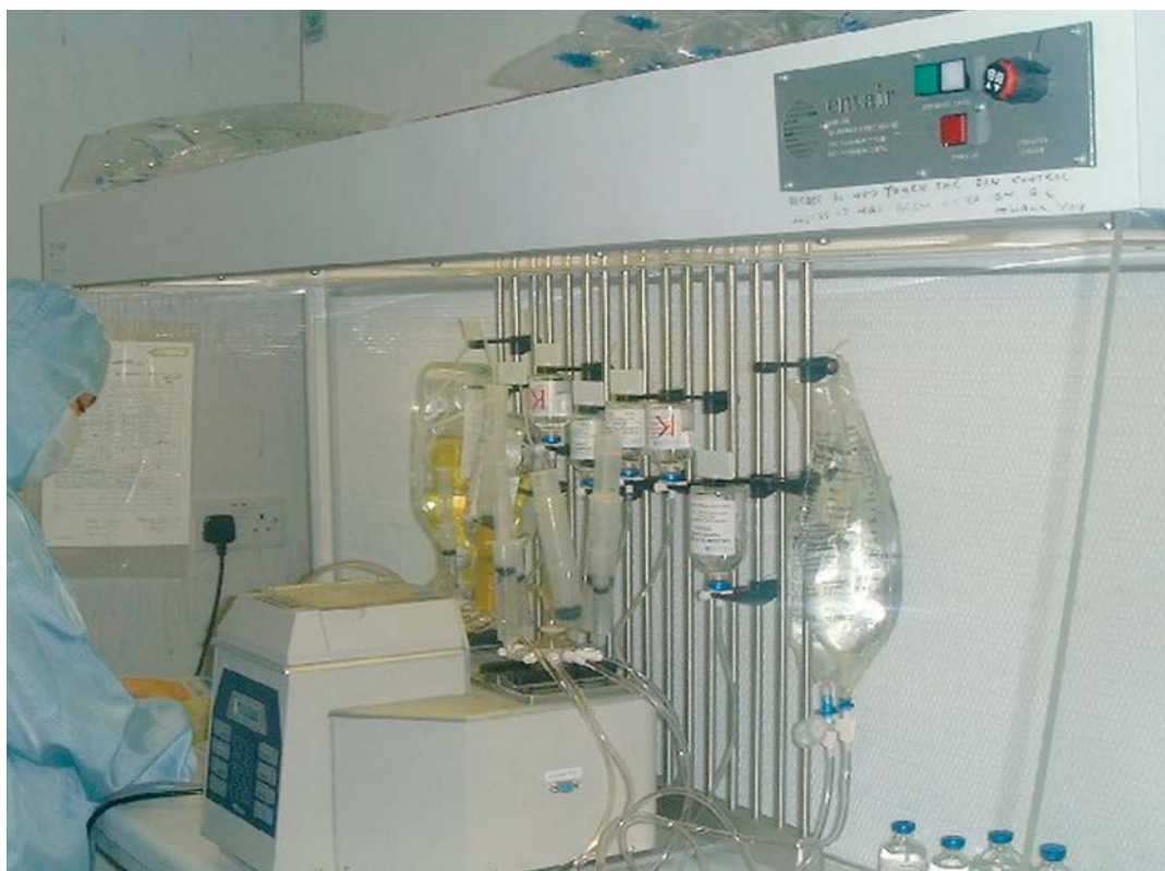
A compounder being used to prepare paediatric parenteral nutrition within the pharmacy aseptic unit at Great Ormond Street Hospital
