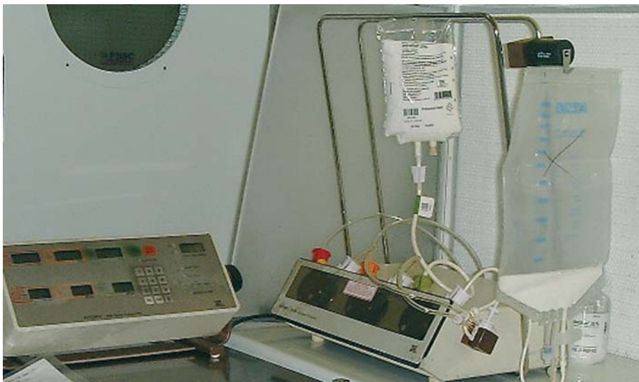
An automix: uses specific gravity to ensure that large volumes of ingredients for parenteral nutrition formulations are mixed correctly
