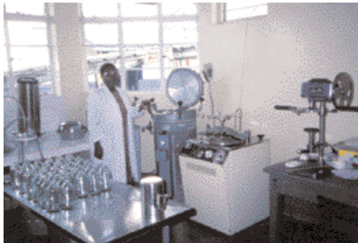
Sterilising glass bottles of intravenous saline in autoclaves in the sterilisation unit
