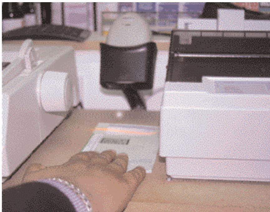
In the Flexiscript ETP pilot, patients are given a paper prescription with a barcode and a serial number on it. Scanning the barcode in a participating pharmacy allows the computer to download details of prescribed items from a central computer
